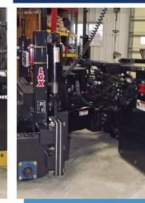
The LGX Burchland Laser Grader is proven to be a reliable attachment for finish grading. You will
